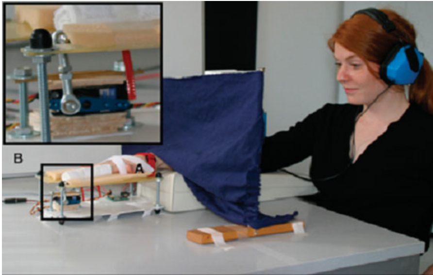
FIG. 1. Testing apparatus. The forearm was placed on a comfortable cushion as an extension of the platform. A: The palm of the subject's hand rested on a padded plastic platform. B: The index finger was surrounded by a soft cotton strap, which attached the finger to the moveable part of the apparatus. The metacarpal joint of the index finger and the joint of the moveable platform arm were positioned exactly vertical to each other. B: The DC motor was placed below the platform. To prevent acoustic information, the subjects wore headphones. The curtain prevented the use of visual information. [Color figure can be viewed in the online issue, which is available at www.interscience.wiley.com .]
